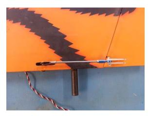
Using a straight edge line up the servo arm with the intended position of the rudder horn. Once marked carefully cut a slot in the rudder to accept the horn, ensure that the horn is in line with the servo arm and that the hole in the horn is positioned over the hinge line. Using a high strength glue like Hysol or Aeropoxy glue the horn into the rudder.
