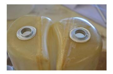
Once dry make up the fuel and vent lines to ensure adequate movement of the clunk so it does not bind in the tank and the vent line goes to the top of the tank.
