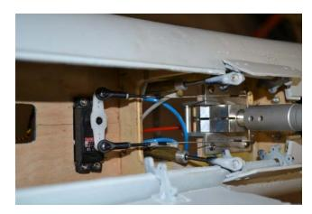
In this build it was decided to use a new mounting tray and make a new servo mount so that the steering cables are a direct pull onto the nose leg.
