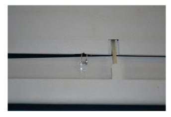
Do this for both servos, it will take some trial and error to get the rod lengths correct for both servos to ensure even travel and no binding.
