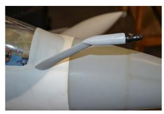
Its best to screw on this piece to the tail of the Mirage prior to fitting the thrust tube as it needs to be screwed from the inside.
