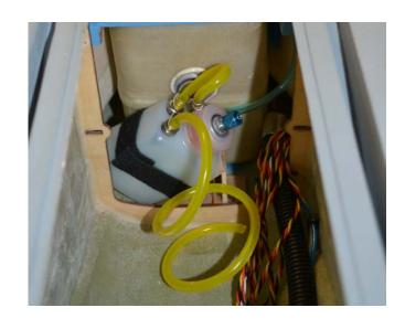
There is ample room in front of the main tank to fit your desired UAT, make a mount as appropriate and fit the UAT.
