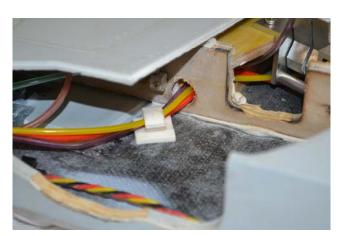
Connect the airlines to the retracts and air brakes. It is a good idea to use a different colour line for each function, these aids in setting up the different functions.
