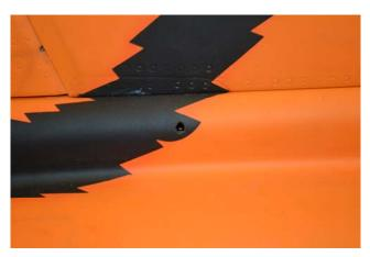
Attach the fin to the fuselage using the prepositioned internal bolt.
