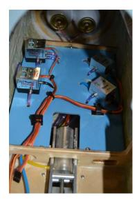
The front mounting tray was used to house the air valves. There are mechanical valves supplied with the kit which are adequate to undertake the air system requirements. In this build we chose to use electronic valves which you will need 3 x 2 way valves and a brake valve.
