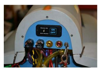
A control panel was made to fit in the forward opening of the turbine compartment.
