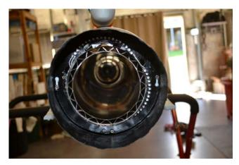
The supplied thrust tube should be good for turbines up to 16 Kg thrust but may deform if larger engines are used.
