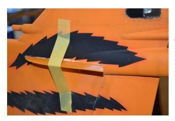
Carefully mark the position of the fences on the top of the fin and cut a small slot. Using hysol or similar glue the fences to the top of the fin.
