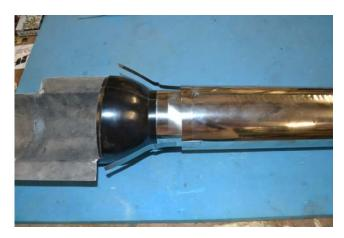
Mount your turbine as per manufacturer's instructions on the turbine rails. It is very important to ensure that the thrust line of the turbine runs down the centre of the thrust tube to avoid hot spots and an offset thrust line.
