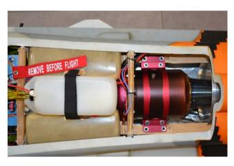
As we were using a larger turbine we added an extra dubro tank located between the two saddle tanks and above the inlet duct, this gave another 700mls of fuel.
