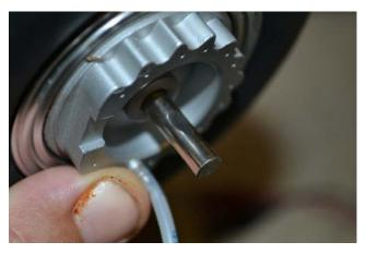
Remove the main undercarriage and check that all bolts are secure and apply loctite if necessary. Remove the axle and grind a small flat on the shaft where the grub screw secures the shaft as an added measure of security.
