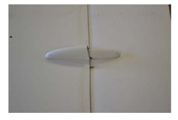
Attach the missile rails to the wings using the bolts supplied. Trial fit the missiles and once satisfied remove as they may be damaged if left attached to the wings. Fit just before flight.
