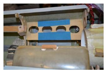
Next install the two saddle tanks in the engine bay using high strength Velcro. It may be required to trim the former to get the tank lines and bung assembly to clear the former. In this build a separate bracket was made to locate the front of the tanks against the former. Once fitted plumb the tanks in your desired method either in series or parallel then to the main forward tank.
