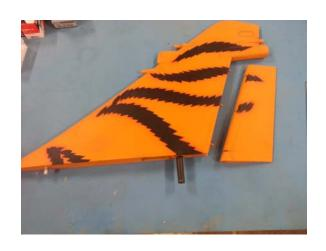
Temporarily fit your chosen rudder servo in the bottom of the fin and mark the opening for the servo arm.
