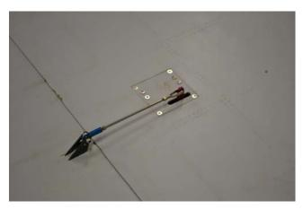
Fit the control rod between the servo and the elevon and ensure adequate movement of the surface.
