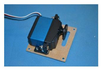
Remove the servo cover for the elevon and with the mounting hardware supplied fit your servo. Given the size of this control surface it is important that a premium quality, high torque servo is used.
