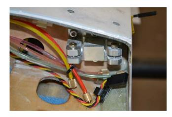
Insert bolts into the wing attachment points
