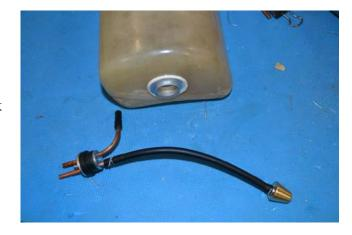
Once satisfied, wash the tank with fuel to ensure all debris is removed. When dry assemble the tank ensuring all lines are lock wired to prevent air entering the system and ensuring security. It is a good idea to pressure test the tanks outside of the model by filling with fuel prior to installation.
